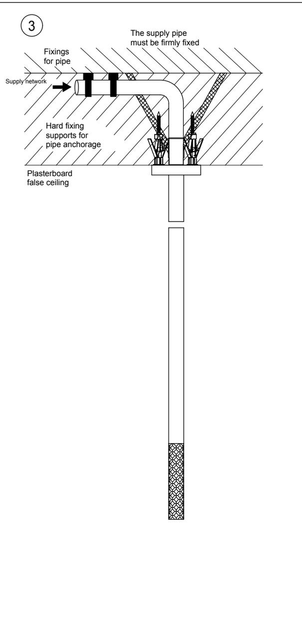
ATTENTION: In the second and third case hard fixing supports are not provided in the box but they need to be realized by the installer during the installation phase
