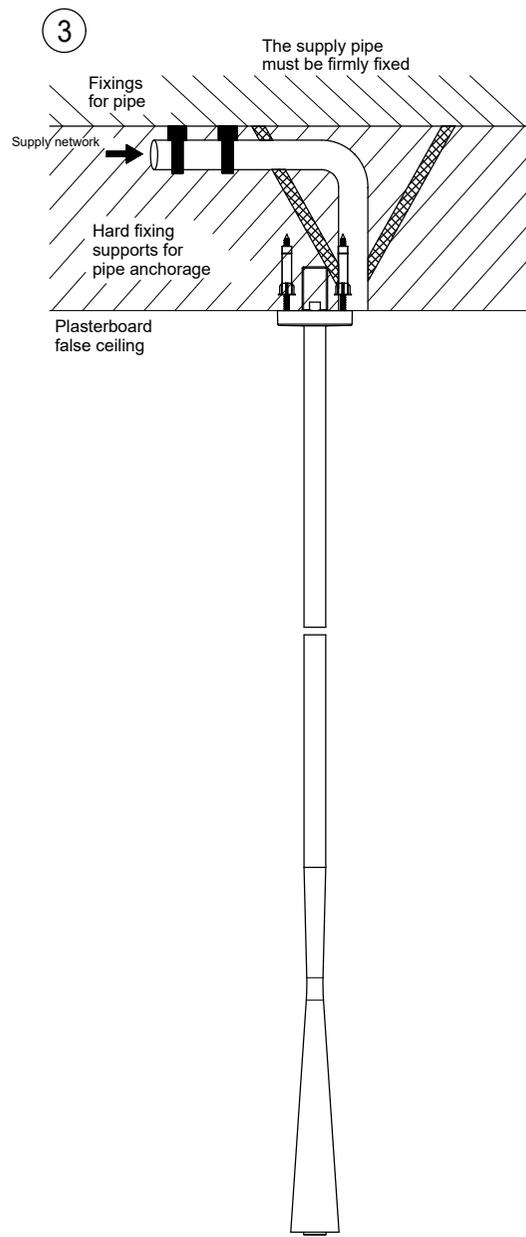
ATTENTION: In the second and third case hard fixing supports are not provided in the box but they need to be realized by the installer during the installation phase
